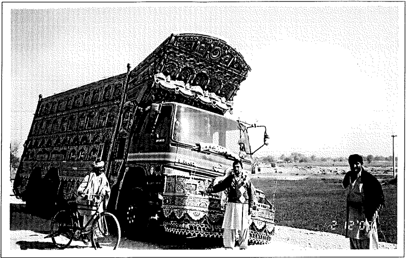
Photograph - 9 A truck stuck up in 'soft' shoulder in the damaged section of N-20
